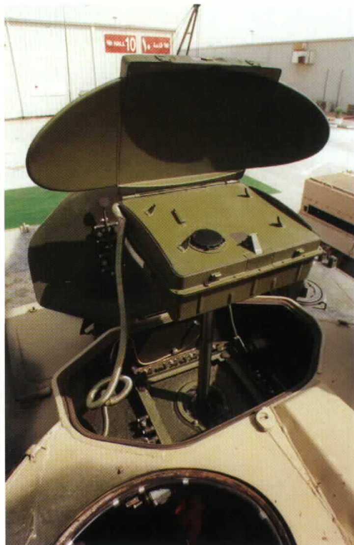
This is a close-up of the RL-133-1 Kredo-1M battlefield surveillance radar. When not in use, it is folded down inside the turret. It has a detection range of 8,000-10,000m against a tank, and 3,000-4,000m against personnel.
