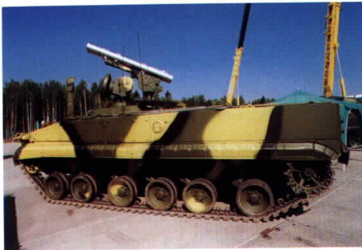
Another view of the 9P157-2 Krizantema tank destroyer with the missile tubes elevated. This missile was designed specifically to destroy advanced main battle tanks like the M1 Abrams that are protected by composite armor. It has a range of 5 kilometers, a speed of 170 m/s, and its 150mm warhead can penetrate up to 800mm of armor.
