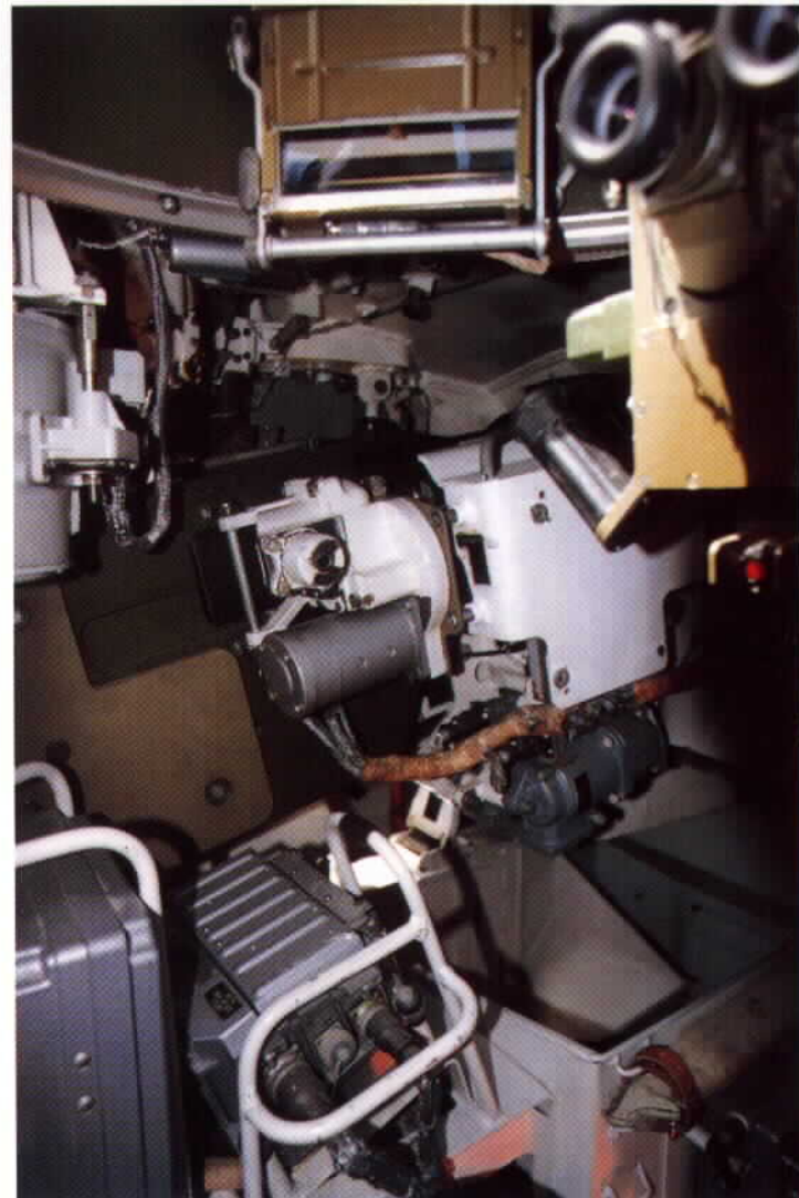
This is the view inside the turret from the commander's seat with the 2A70 gun breech evident in the center.
