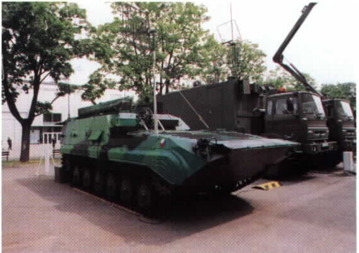
The extended hull BMP used for the Snezhka is also being used for other special purpose vehicles. The AMB-S is a mobile communication relay station used in BMP-2 mechanized battalions to interconnect command posts and other communication sites. Besides carrying a DTP-40 tactical switching set, it also carries a R-150S and R-1325 radio complex.
