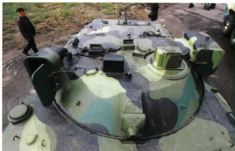
This overhead view of a PRP-4M turret show the distinctive features of this type, including the two electro-optical sensor ports on either side of the turret, and the hatch at the rear of the turret which hinges open to permit a small Kredo-1 battlefield surveillance radar to deploy. The vehicle's only armament is a single PKT machine gun for self-defense in the mount at the front of the turret.
