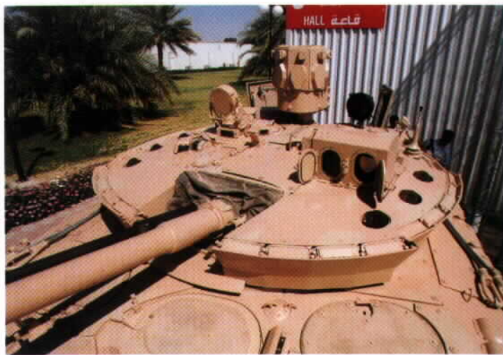
This overhead of the BMP-3 turret with Arena shows the explosive panels stowed vertically around the turret sides.
