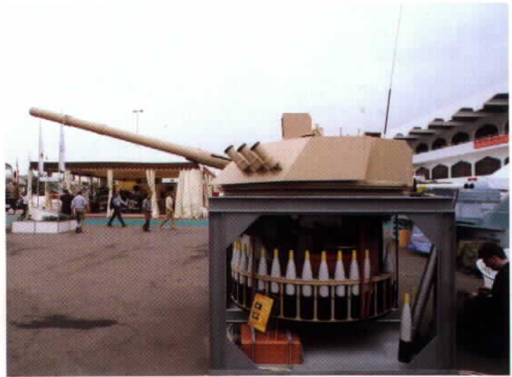
The BMP-3M may eventually be fitted with a new welded turret, shown here in prototype form at an exhibition for the UAE Army in 1998.
