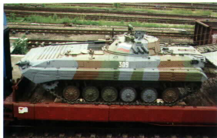
This rear view of the PRP-4M shows its similarity to the basic BMP-1 chassis. However, there are no firing ports on the hull side. The camouflage pattern on this vehicle is typical of local improvisations which have become more common in the Russian Army in the 1990s.
