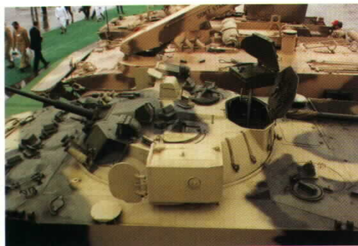
The two boxes on either side of the turret contain electro-optical sensors including the 1PN61 image intensification night vision sensor with a laser illuminator, and the 1PN71 is a thermal night vision sight. The Kredo-1M battlefield surveillance radar is erected.
