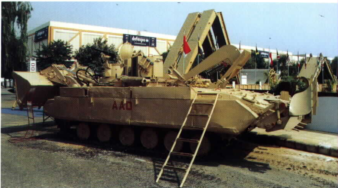
India is building a wide variety of BMP derivatives for special purpose applications. This is the Namica, a tank destroyer that is designed for India's indigenous Nag anti-tank missile. The Nag (Snake) missile is fired from the elevated armored box launcher seen above the vehicle which also contains the guidance package. (Wojciech Luczak)
