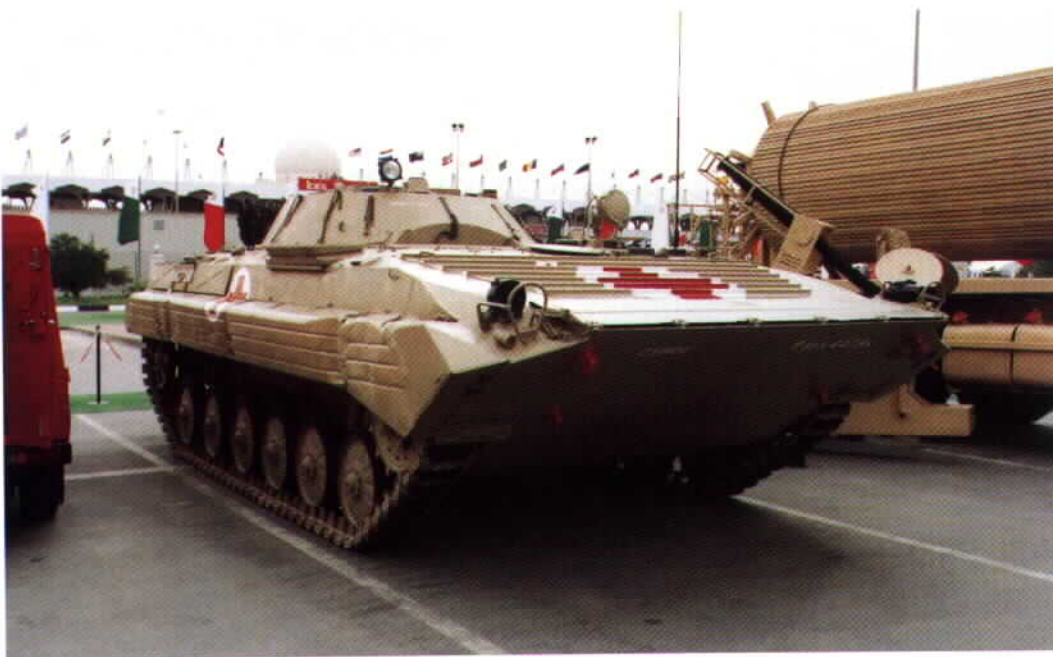
The AERV is a dedicated armored engineering reconnaissance vehicle. The gun is removed, and the space used for electro-optical sensor equipment. The devices on the side are minefield markers which are used to mark cleared lanes created by the AAO vehicle. (Wojciech Luczak)
