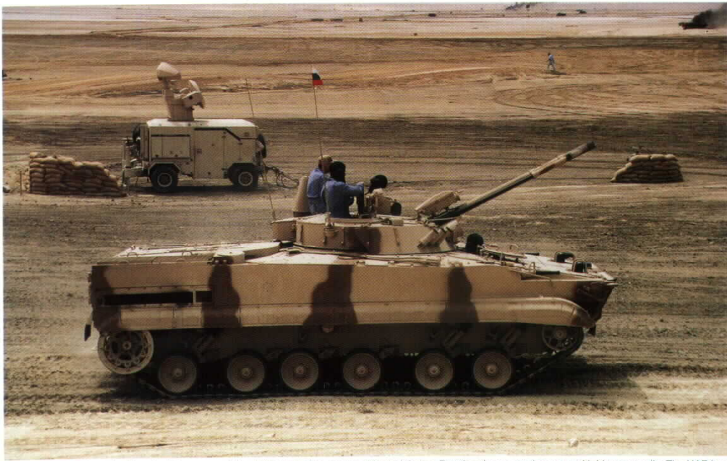
A UAE BMP-3 on the Maqatra firing range of the UAE Army. The crew in this vehicle is a Russian demonstration crew with blue coveralls. The UAE has had some problems with the BMP-3 in sand, and the Russians had to develop an additional ring for the drive sprocket to prevent the tracks from shedding.
