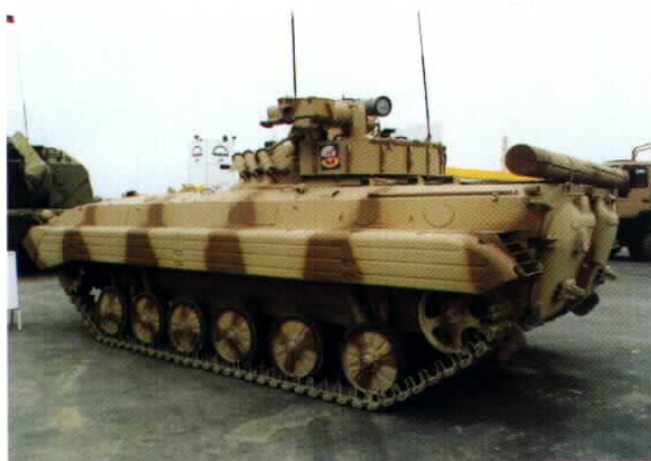
This rear view of the current BMP-2 export vehicle shows one of the key features of the modernization package, the new AG-17 30mm grenade launcher on the left rear of the turret along with an ammunition tray curving along the rear of the turret. The Russian Army has shown much more interest in automatic grenade launchers like these after its experiences in urban warfare in Chechnya.
