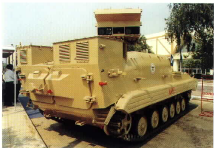
This rear-view of the Namica shows the enlarged superstructure at the rear, along with the vents for the added electrical equipment. (Wojciech Luczak)
