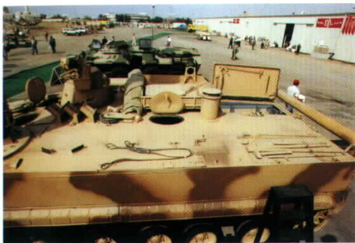
The left side deck on the Beglianka is plain since the crane rests here when not in use. Note the six smoke mortars mounted along the centerline of the vehicle towards the front.
