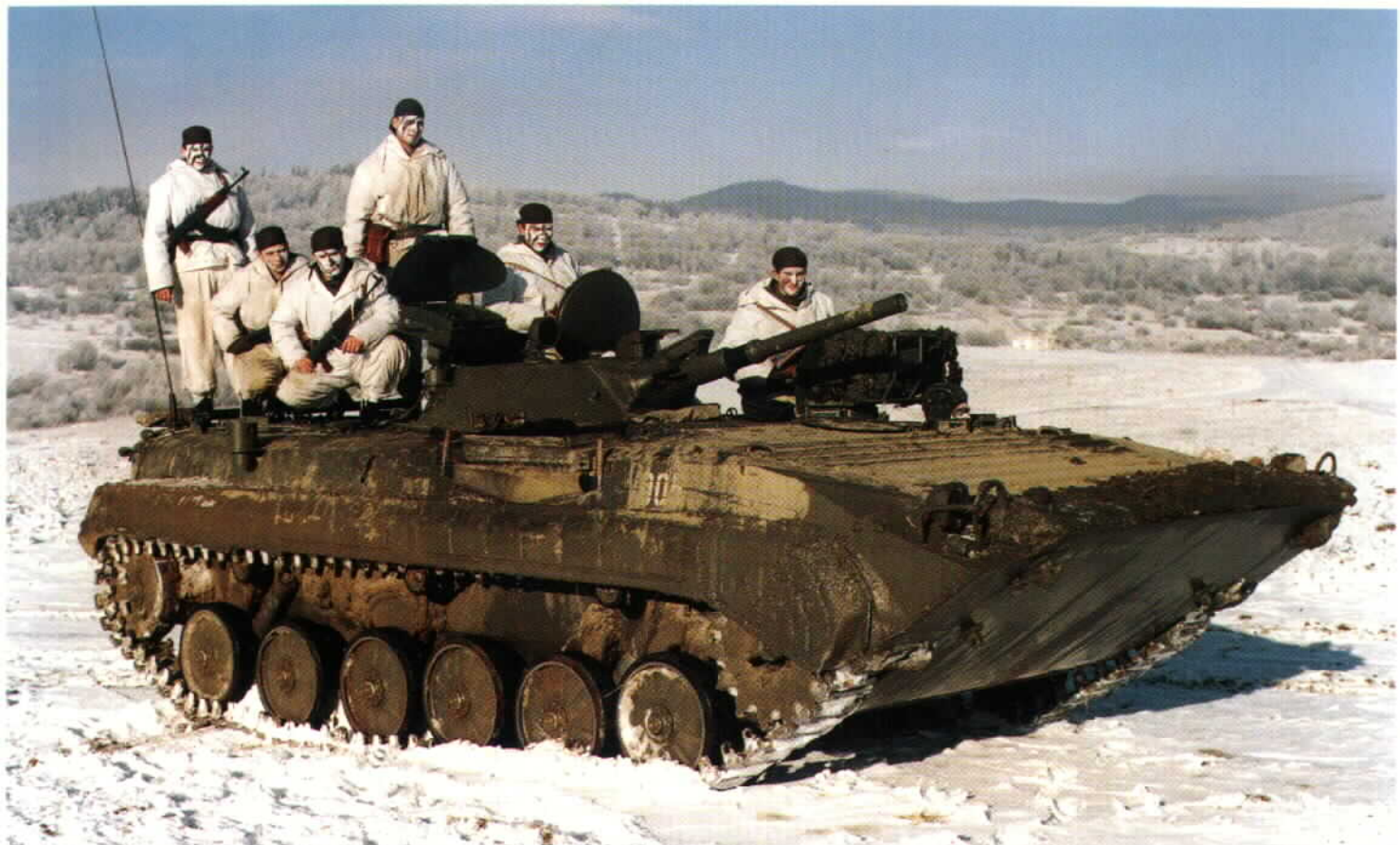
Another view of a BPzV of the Czech 4th Rapid Deployment Brigade. The electro-optical day/night sight is in the pod evident immediately below the 73mm gun barrel. (Josef Spurny)
