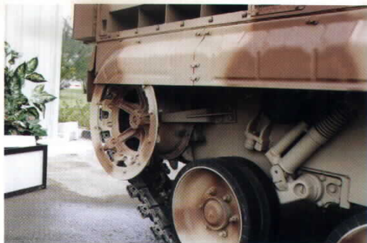
This is a useful comparison on the detail differences between the UAE vehicles and the early production Russian vehicles. The UAE vehicles have a large ring added around the drive sprocket to prevent track shedding, a recurrent problem in the local sandy conditions. Also note the use of improved, reinforced bump stops on the hull side.
