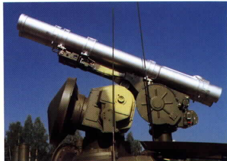
This close-up shows the twin launch tubes on the Krizantema launcher. The vehicle stows a total of 15 missiles in its reload cell and the launcher is reloaded automatically. Behind it is the radar sensor used both to acquire targets at long range and to guide the missile.
