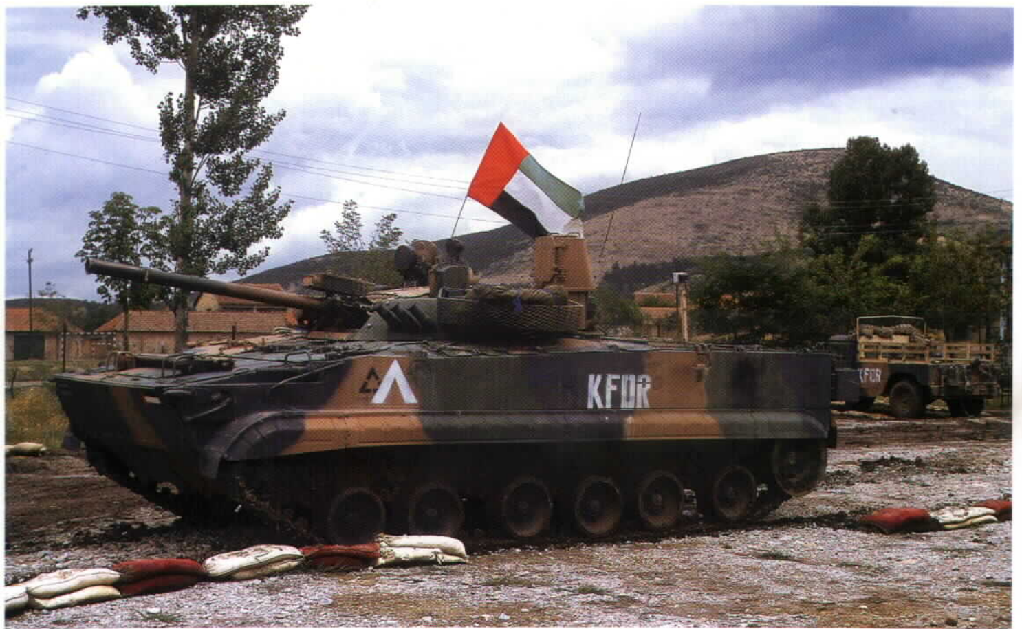
The BMP-3 in the KFOR detachment have had some modifications, notably the addition of stowage racks on the sides and behind the turret for crew gear. (Yves Debay)
