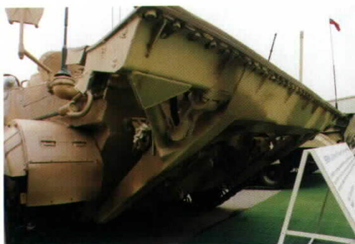
This is a detail view of the dozer blade fitted to the front of the Beglianka. Although it can be used for normal bulldozer operations, it is most often used to anchor the vehicle when using the winch to recover bogged-down vehicles.
