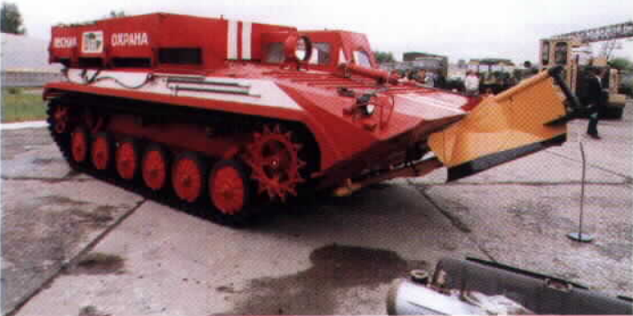
The availability of surplus BMP-2 chassis has led to their modification for civilian roles. This particular example is intended for forest fire fighting units with a work platform on the rear for equipment, and a plow for creating fire breaks.
