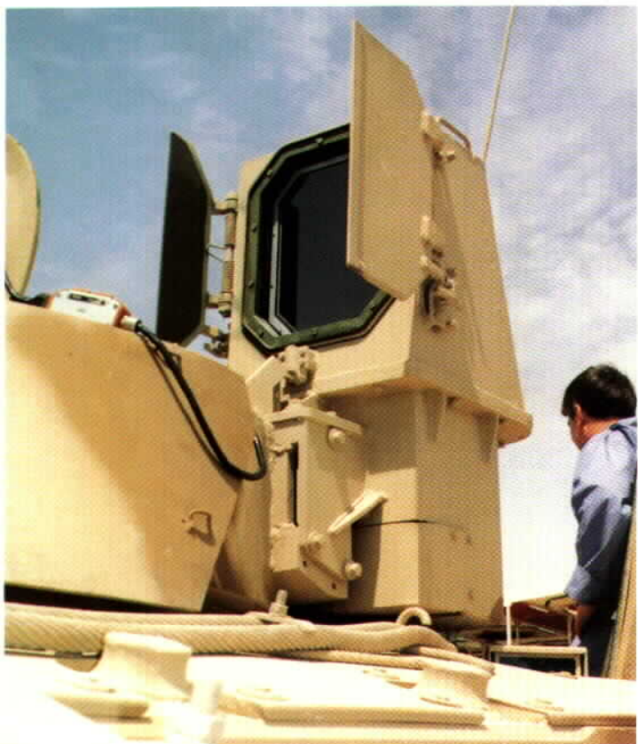
On the late production UAE BMP-3, there is an armored cover over the 1D16-2 laser range finder. To the lower left is the gunner's 1K13-2 day/night sight, and a smaller 1PZ-10 high elevation optical sight for engaging aerial targets.
