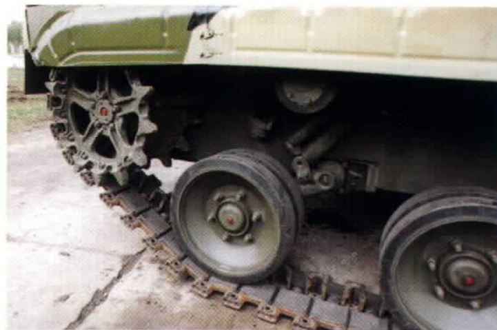
A useful detail view of the rear portion of the suspension on the right side of a standard production Russian vehicle. This gives a good view of the track, the drive sprocket, and the suspension arms.
