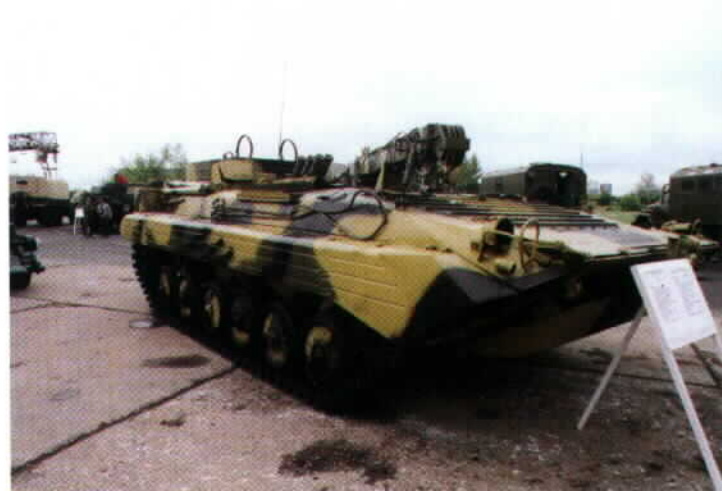
Another view of the BREM-2 shows the jib crane and the work platform mounted on the rear of the vehicle. As in the case of the BMP-2, it is fitted with the wider mud guards which provide added buoyancy in water.
