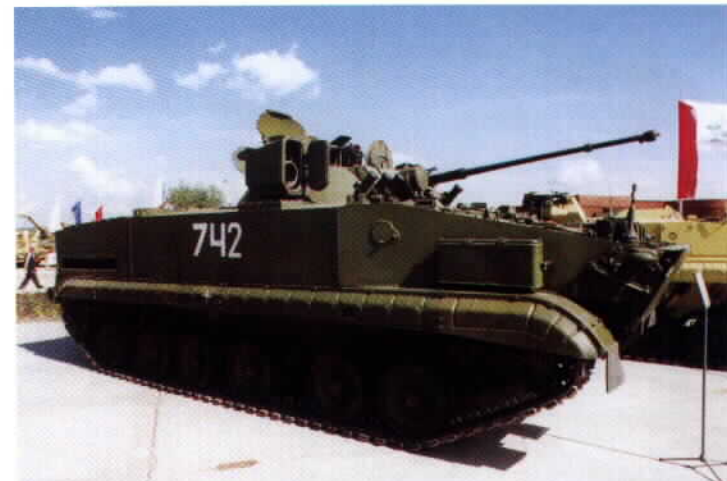
A BRM-3 on display in Russia near Nizhni-Tagil with a tactical number marking. There are very few of these vehicles in service, mainly in Siberia. This vehicle does not have the front corner machine guns like the normal BMP-3, but has an additional gun port on the front panel.
