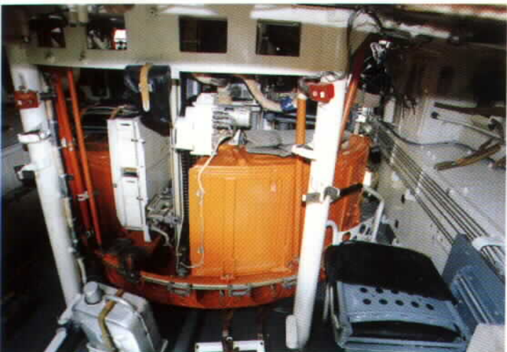
This is a view of the turret basket inside the BMP-3 taken from the rear of the vehicle as it appears when first crawling into the BMP-3 through the rear doors. The red/orange paint is typical of BMP-1/-2/-3 turret baskets, and is used to warn troops to keep their hands and equipment away from moving parts. The autoloader holds 22 rounds of ZOF17 and ZOF32 high explosive projectiles, while an additional 18 HE rounds and six 9M117 guided missiles are stored elsewhere in the hull.
