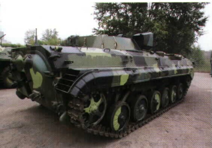
This rear view of the PRP-4M shows its similarity to the basic BMP-1 chassis. However, there are no firing ports on the hull side. The camouflage pattern on this vehicle is typical of local improvisations which have become more common in the Russian Army in the 1990s.
