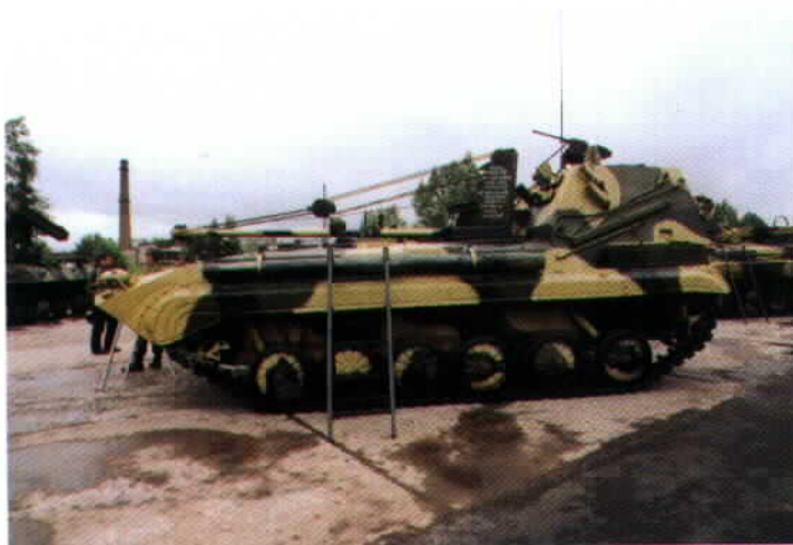
With the BMP-2 chassis still in production in Russia, some new specialized versions have been developed. One of the most recent is the RM-G tracked recovery vehicle. This is fitted with a 3 ton KU-3 crane, and has a variety of other repair equipment on board.
