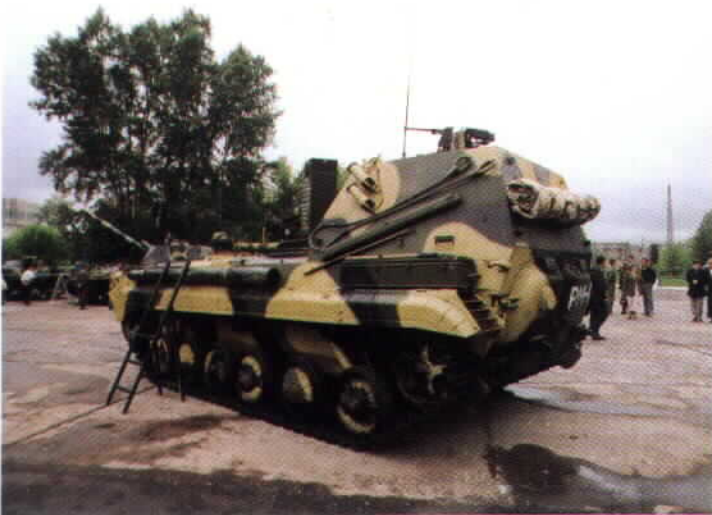
A rear view of the RM-G on display at an arms exhibit in Omsk in 1998 provides a good view of the added superstructure at the rear.
