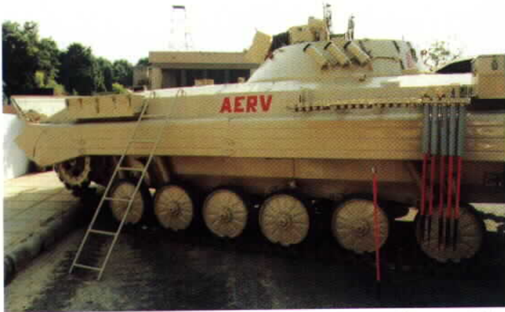
The AERV is a dedicated armored engineering reconnaissance vehicle. The gun is removed, and the space used for electro-optical sensor equipment. The devices on the side are minefield markers which are used to mark cleared lanes created by the AAO vehicle. (Wojciech Luczak)
