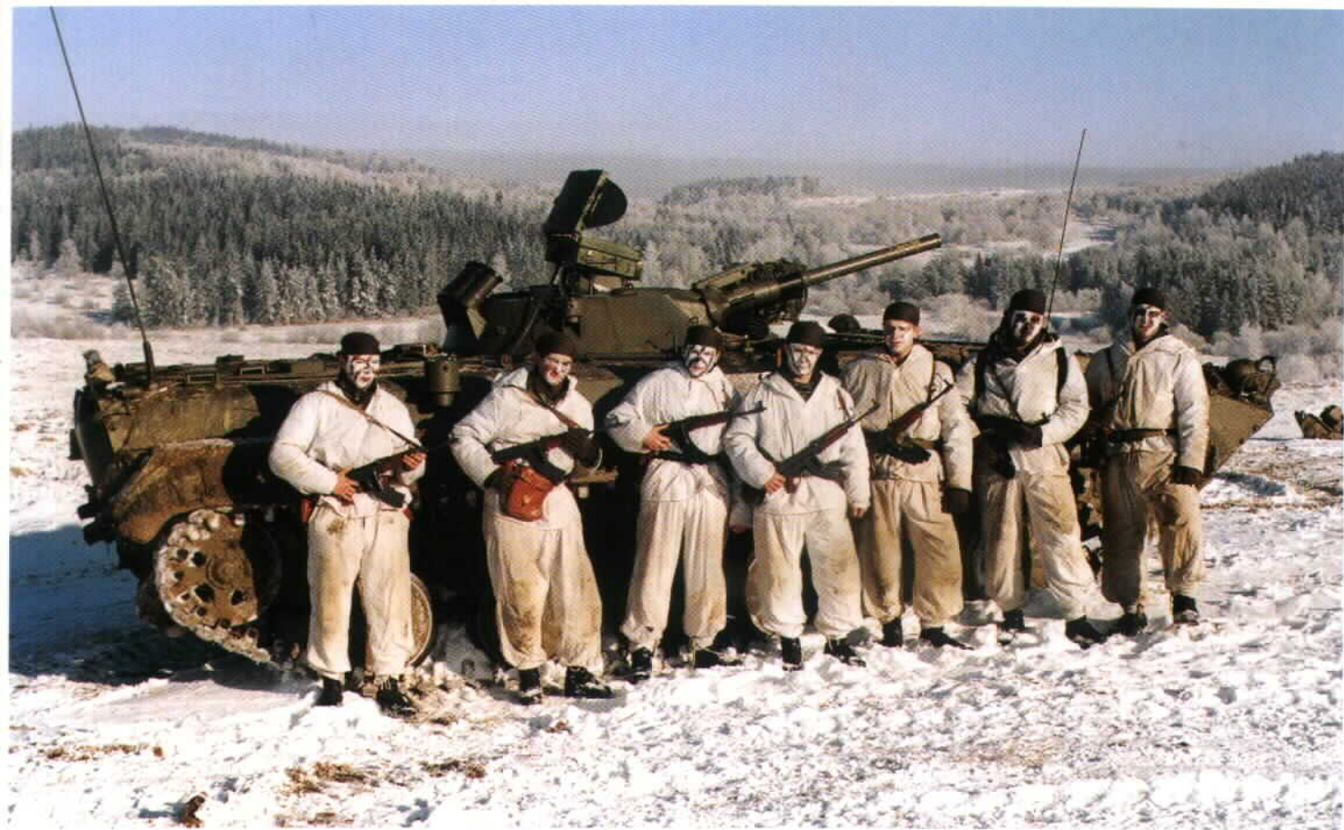
The Czech Army developed its own equivalent of the Russian BRM-1 reconnaissance vehicle, called the BPzV. This is basically a BMP-1 with added radar and electro-optical sensors. The PSNR-5K radar can be seen above the turret. This is a vehicle of the Czech 4th Rapid Deployment Brigade. (Josef Spurny)
