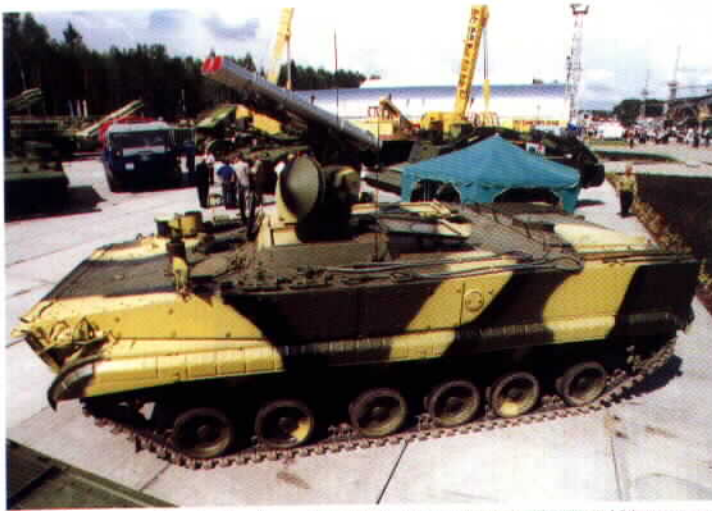
The competitor to the Kornet tank destroyer is the 9P157-2 Krizantema tank destroyer. With the collapse of the Russian defense budget, Russian firms are much more dependent on export sales for survival. So now, Russia often produces weapons for the export market that are not sold to the Russian Army. This vehicle is highly automated and has a crew of only two: a driver and a gunner.
