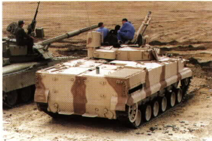
A good overview of a UAE BMP-3 sitting next to a Russian T-80U at Maqatra. The aluminum can on the back deck is the stub casing of a 100mm ammunition round that has been ejected from the gun through the turret hatch.
