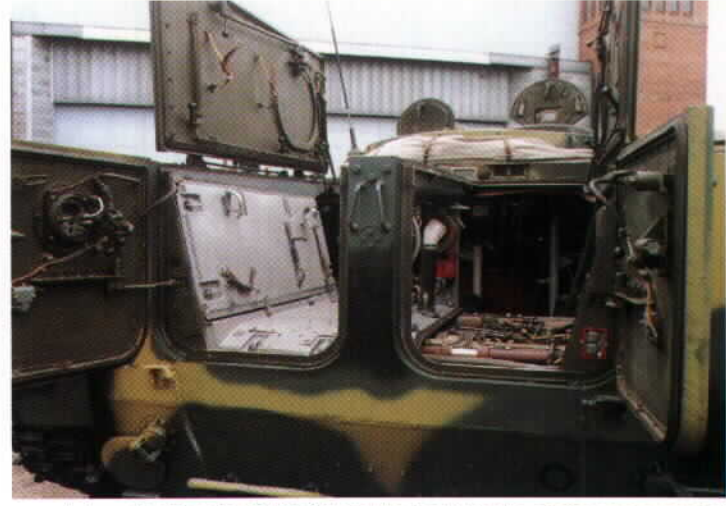
A view of a Russian BMP-3 from the rear with the engine access panel open shows how cramped the engine compartment is under the floor.
