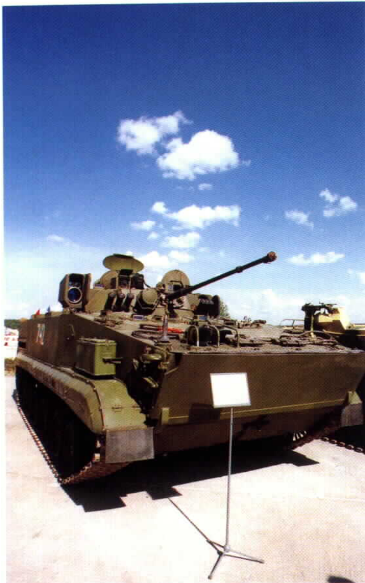
One of the less often seen variants of the BMP-3 family is the BRM-3 Rys (Fox). This is a scout version of the vehicle, and lacks the 100mm gun. It is manufactured at the Rubtsovsk Machine Building Plant in the Altai region of Russia rather than the Kurgan plant that manufactures most BMP-3s.
