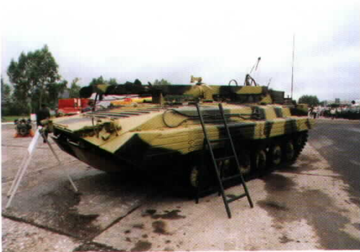
One of the most seldom-seen BMP variants is the BREM-2 armored recovery/maintenance vehicle. This is fitted with a 1.5 ton jib crane and a winch for work on light armored vehicles. This vehicle is in service with a Russian unit in Siberia and is painted in a local scheme of sand/green and black over the usual dark green.
