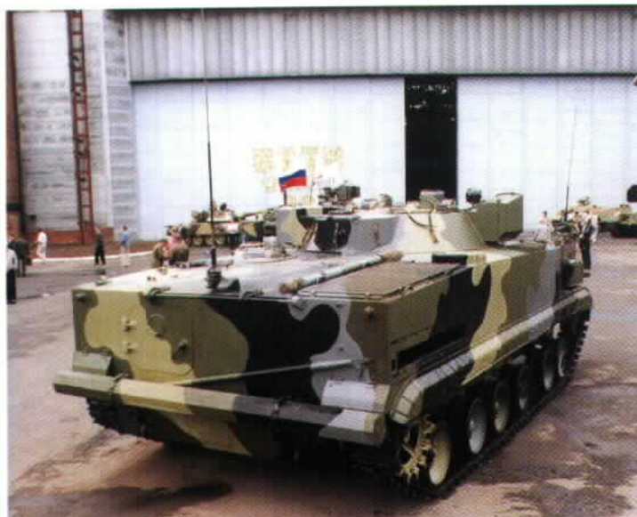
An overhead view of the Omsk BRM-3 shows that it lacks the opening doors on the rear deck. The tube on the rear deck is for stowing a long radio antenna.
