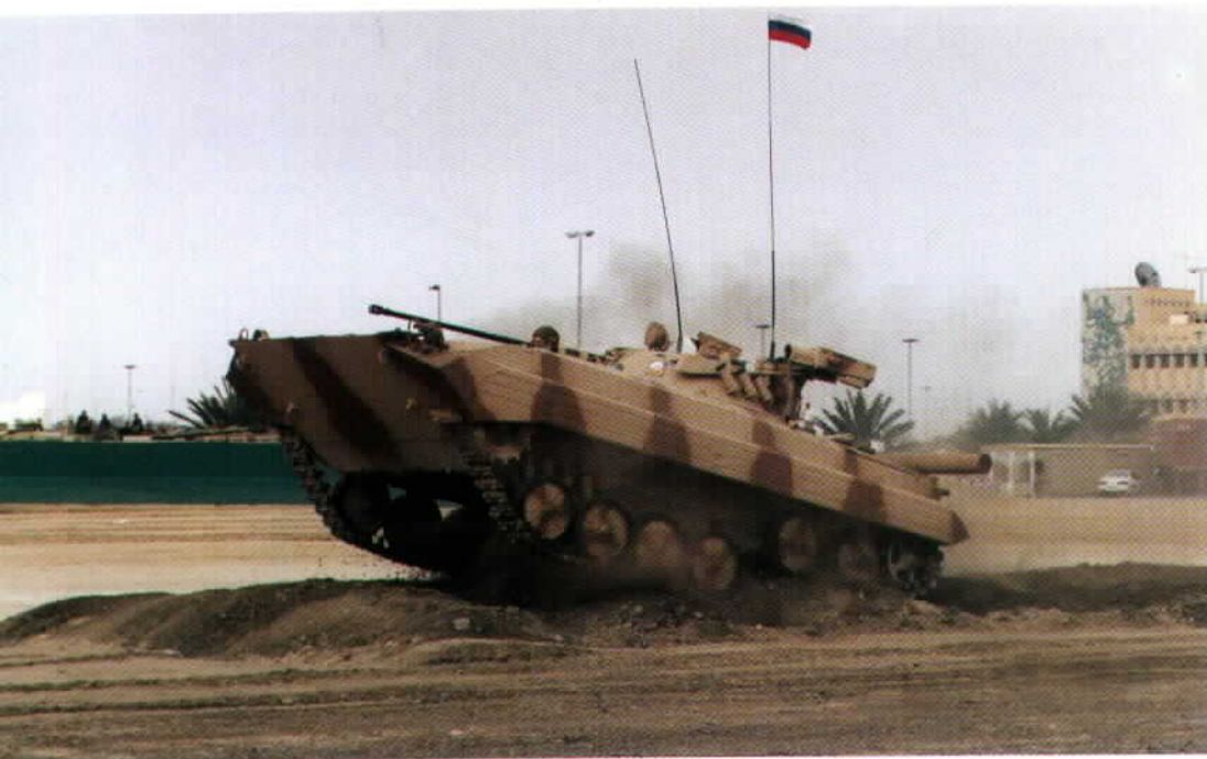
The modernized BMP-2 can be fitted with the updated UTD-23 turbocharged diesel engine which gives it better performance as demonstrated here on an obstacle course.
