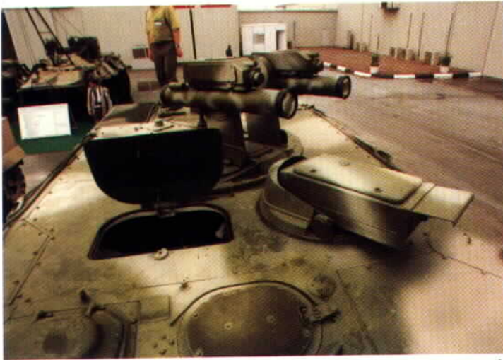
A close-up of the gunner's sight on the 9P162 Kornet tank destroyer. It traverses along with the turret.
