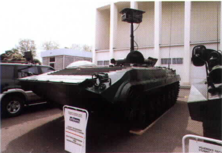
The BMP-1 is widely regarded as being obsolete, so the Czech Army has been considering rebuilding some of these vehicles for other roles. This is one proposal, a light artillery reconnaissance vehicle on a modified BMP-1 chassis. The gun is plated over, an electro-optical sensor package is fitted on an elevating mast. This is intended as a cheaper alternative to the Snezhka.
