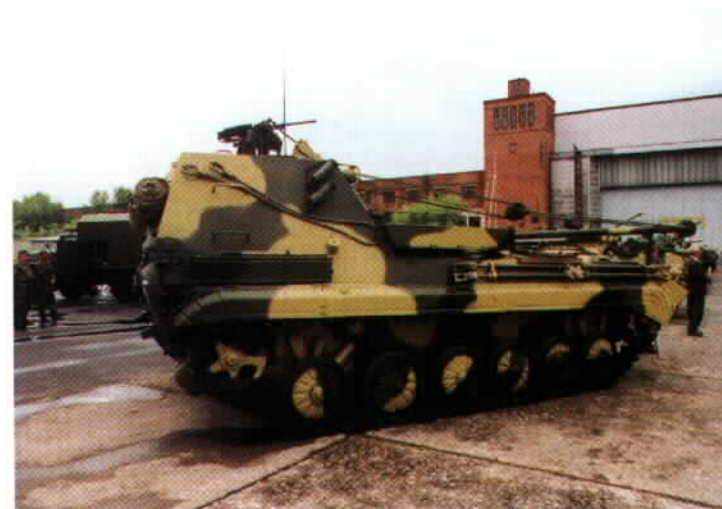
This side view of the RM-G shows the higher superstructure of this recovery variant. This is intended for heavier duty tasks than the older BREM-2 design.
