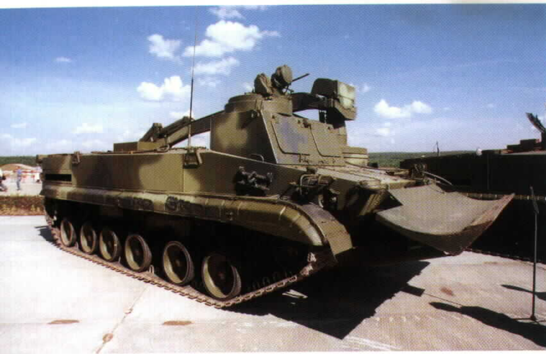
One of the rare pieces of equipment developed for the BMP vehicles is the KMT-10 mine rake. Since the BMP is too light to push a mine roller, this configuration is used to dig in and push mines out of the way.
