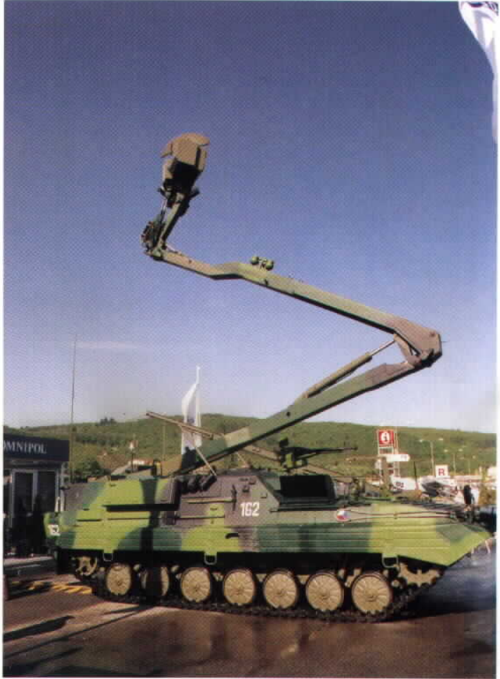
The Czech Republic also has manufactured the BMP under the local designation of BVP. One of the most sophisticated new variants is the Snezhka, a dedicated artillery forward observer vehicle. The elevating mast is fitted with an electro-optical sensor and radar, which can be elevated over trees or other obstructions for long-range observation. The large crew compartment in the rear has led to the extension of the hull.
