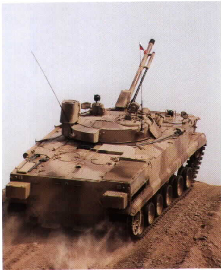
A good overview of a UAE BMP-3 shows some of the other changes on the late production batches including the additional stowage bin on the turret rear, and the two stowage boxes on the hull rear. The UAE Army vehicles are often fitted with an externally mounted fire extinguisher on the hull side.
