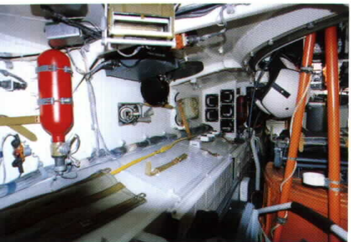
This is a view down along the space on the left side of the hull. There would normally be ammunition stowed in the forward area.
