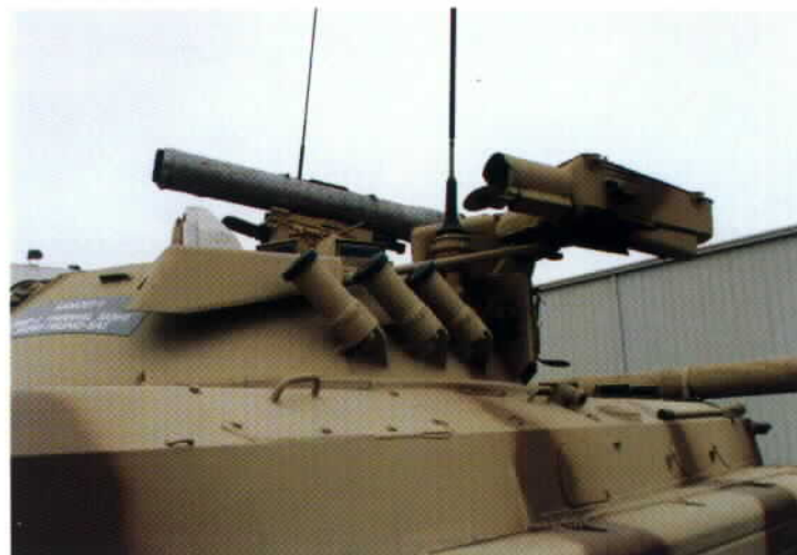
This is a close-up of the AG-17 grenade launcher on the modernized BMP-2. The bar below is an articulation arm for the grenade launcher to permit the turret crew to elevate the weapon.
