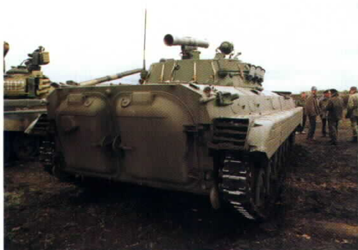
A BMP-2 with a Russian motor rifle unit in Siberia in 1997 showing the two access doors at the hull rear. These double as fuel cells.
