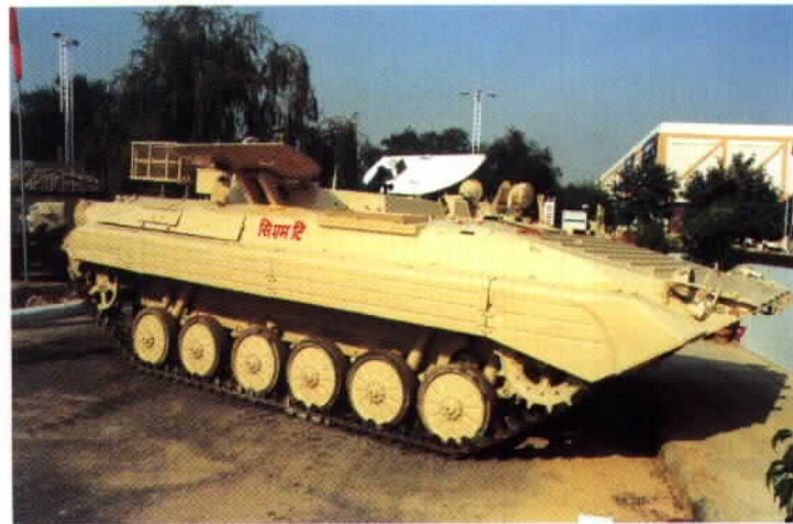
India is also beginning to manufacture a dedicated 120mm mortar derivative of the Sarath. As seen here, the mortar is contained in the center of the vehicle instead of the usual turret, with two hinged doors above. (Wojciech Luczak)
