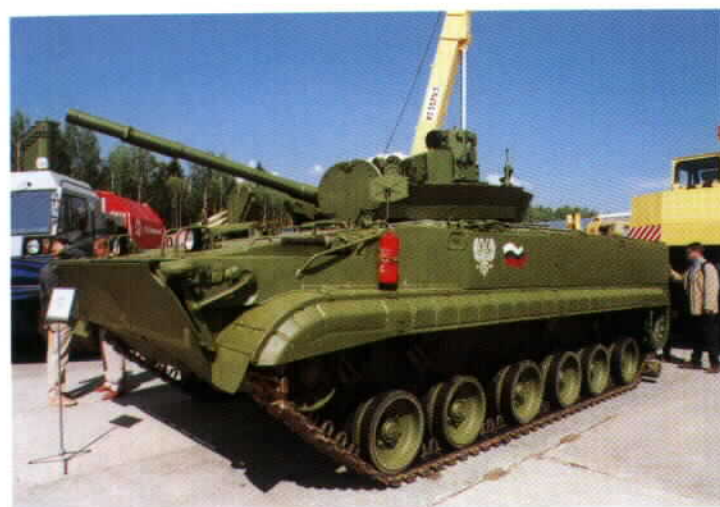
This is another example of the Arena ADS, fitted to a Russian BMP-3.
