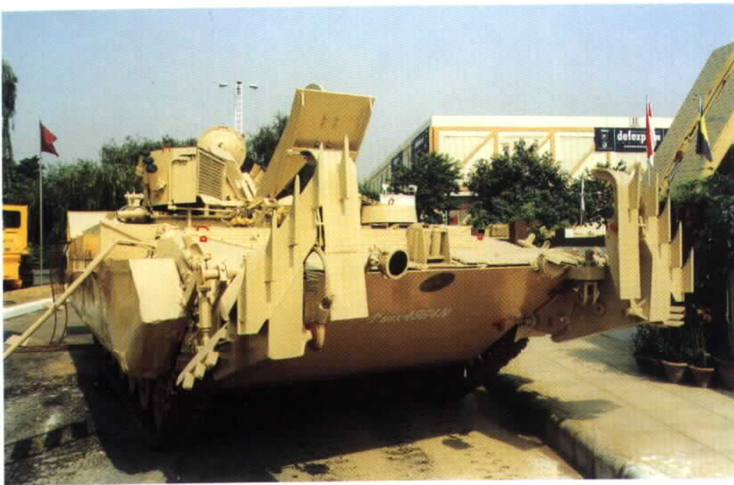
This front-view of the AAO shows the locally-developed mine rakes. This dig into the ground, and push aside the exposed mines rather than detonating them. (Wojciech Luczak)
