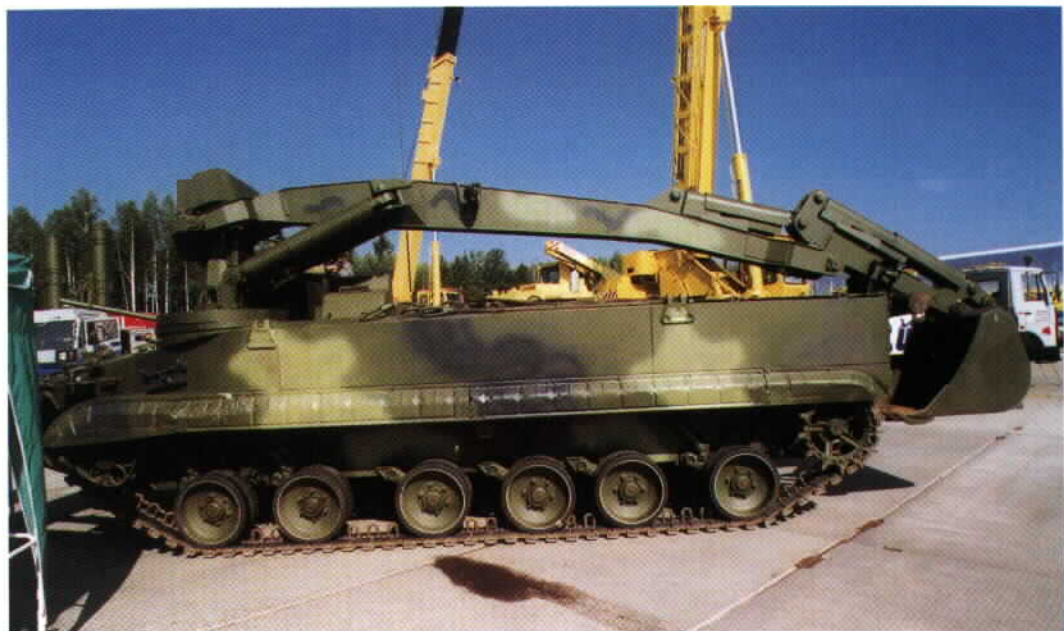
This is the DZM Vostorg combat engineer vehicle developed at the Murom plant. It includes excavating equipment and other devices for combat engineers including a dozer blade.
