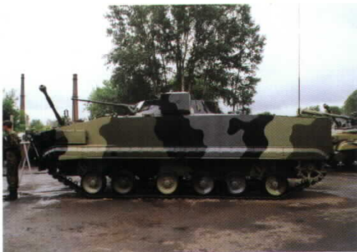
One of the few BRM-3 in service, on display in the Siberian military district near Omsk. The paint scheme is also a local variant, consisting of sand-green, gray and black over the usual dark green. Although superficially similar to the BMP-3, the BRM-3 is almost completely different from the fender line upwards. The BRM-3 uses a higher hull, and a completely different turret.
