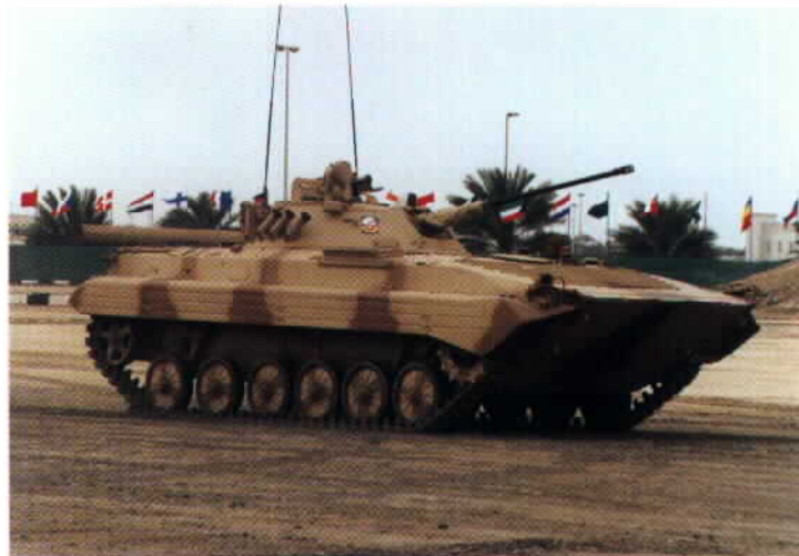
Although the BMP-3 is now in production at Kurgan, the BMP-2 is still being offered for sale. This is the current configuration of the BMP-2 for export, shown in desert camouflage during a display to the United Arab Emirates in 1997. The insignia on the turret is the Rosvooruzhenie export organization's crest.
