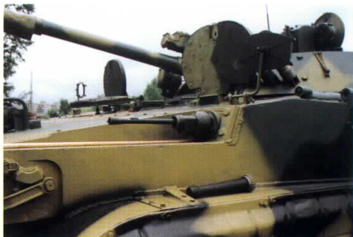
This is a detail view of the forward hull PKT machine gun. The plastic cover for the gun can be seen below.
