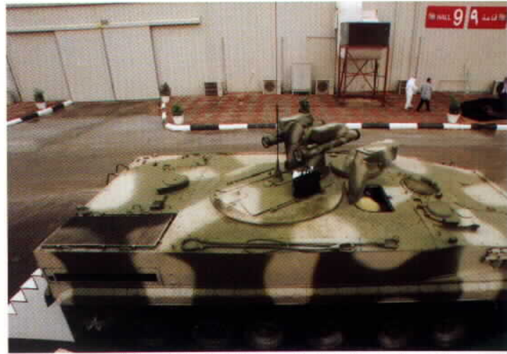
An overhead view of the 9P162 Kornet tank destroyer shows its general features. Below the turret is a twelve round revolver system for rapid reloading of the missiles.
