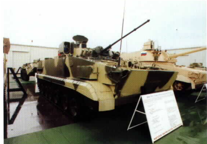
Another view of a BRM-3, this time on display in the UAE in hopes of attracting export interest. The BRM-3 is intended to replace a variety of scout vehicles including the PT-76 light tank; PRP-3, and PRP-4 artillery scouts and the BRM-1 reconnaissance vehicle. This one is finished in the standard Russian camouflage scheme.
