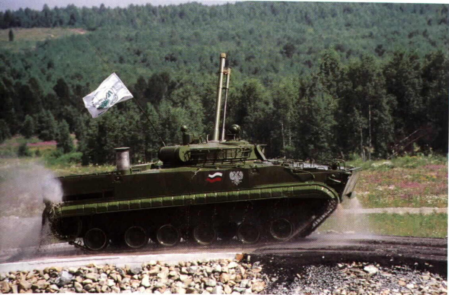
The BMP-3F after having emerged from a water obstacle, with the engine air intake snorkel in raised position. In ocean operation, the larger snorkel mounted on the turret would be fitted in this location.
