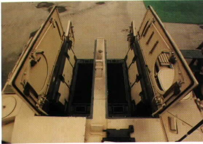
This is a view looking into the rear compartment with the access doors open. The vehicle's UTD-29 engine is mounted under the floor. This is pretty much wasted space, as if the crew uses it for stowage, it interferes with entry and exit from the vehicle.
