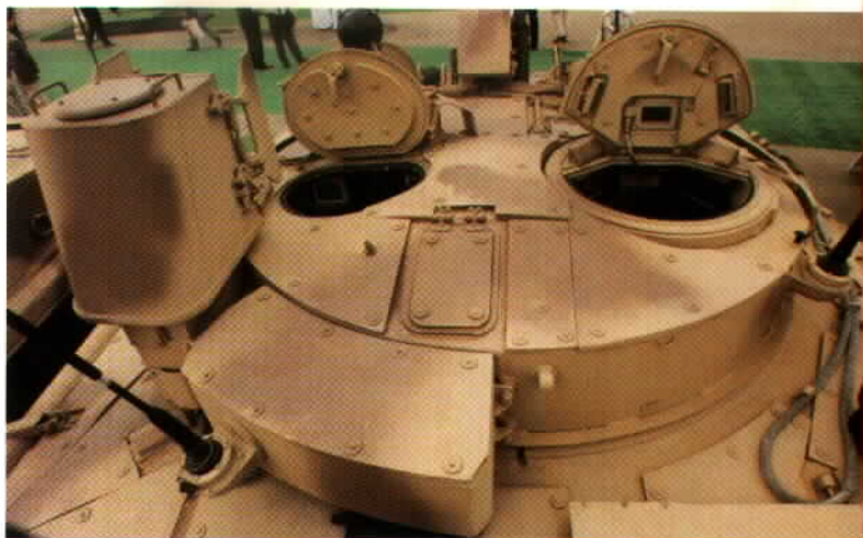
This rear view of the turret of a UAE BMP-3 shows the added stowage bin, the Namut thermal imaging sight, and the added roof appliqué armor.
