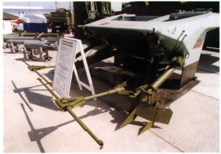
One of the rare pieces of equipment developed for the BMP vehicles is the KMT-10 mine rake. Since the BMP is too light to push a mine roller, this configuration is used to dig in and push mines out of the way.
