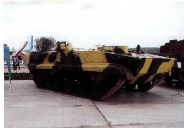
The launcher and radar guidance package on the 9P157-2 Krizantema fold inside the vehicle when not in use. The device on the hull side is a reloading system which allows two men to reload the long missile tubes without the need for a crane or other specialized equipment.
