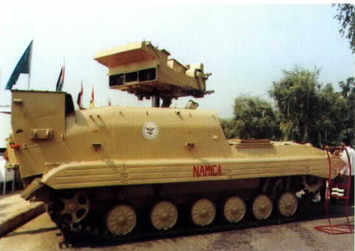
India is building a wide variety of BMP derivatives for special purpose applications. This is the Namica, a tank destroyer that is designed for India's indigenous Nag anti-tank missile. The Nag (Snake) missile is fired from the elevated armored box launcher seen above the vehicle which also contains the guidance package. (Wojciech Luczak)
